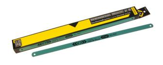
Features & Benefits  $\sim$  Virtually unbreakable with superb cutting power and flexibility  $\sim$  Shatterproof HSS Bi-metal construction  $\sim$  Length: 300 mm / 12\"  $\sim$  TPI (teeth per inch): 32  $\sim$  Contents: 25 hacksaw blades
